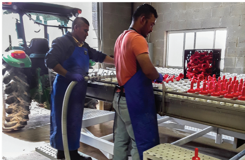
Operator friendly controls for easy pan rotation. Pans can be locked in multiple positions for easy bottle filling, feeding, cleaning and draining.
